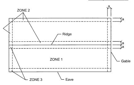
Note: Dimension (a) is defined as 10% of the minimum width of the building or 40% of the mean height of the roof, whichever is smaller, however, (a) cannot be less than either 4% of the minimum width of the building or 3 feet.
