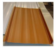
A standing-seam metal roof consists of metal panels running vertically on the roof deck. Each panel has two seams that stand up vertically and are fastened together to seal the joint and keep the elements from penetrating. This design prevents screws from being exposed to the elements which is beneficial for a lower pitched roof, if installed properly.
